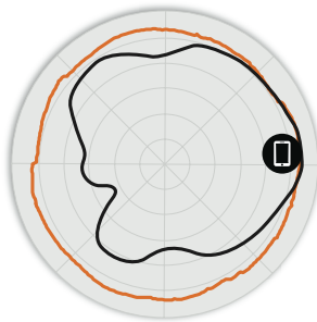
Figure 3 - T310d 5GHz Azimuth Antenna Patterns
